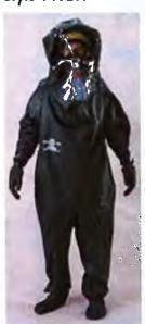
This suit is constructed of nylon and is put together with sewn seams – a very low-cost alternative for the training environment. Suit has rear entry, expanded back, 20 mil. PVC faceshield, single storm flap, gloves, 2 exhaust ports and attached sock boots.
