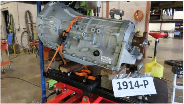
TRANSMISSION REMOVAL AND REPLACEMENT (6.00 LABOR HOURS)
