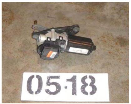
WIPER MOTOR REMOVAL AND REPLACEMENT (0.50 MAN HOURS)
