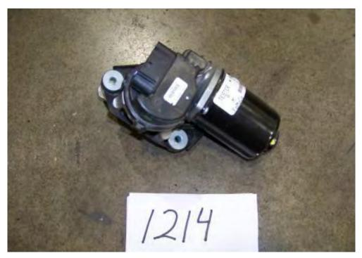
WIPER MOTOR REMOVAL AND REPLACEMENT (0.50 MAN HOURS)
