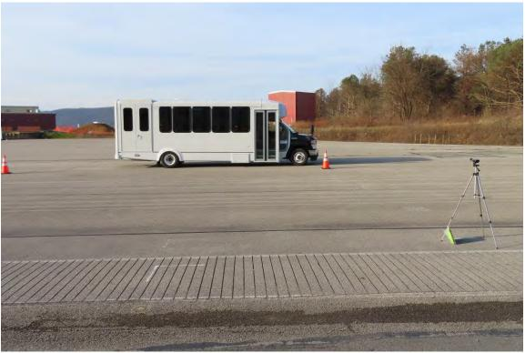
**TEST BUS UNDERGOING EXTERIOR NOISE TESTING**
