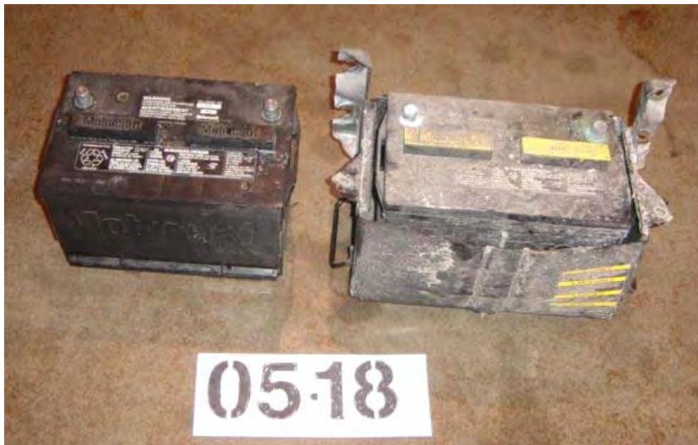
BATTERY REMOVAL AND REPLACEMENT (1.00 MAN HOURS)
