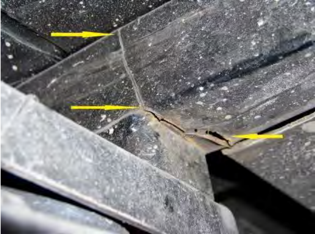
NUMEROUS FLOOR FRAME MEMBERS ARE CRACKED FORWARD & REAR OF THE REAR AXLE (2,171 TEST MILES)
