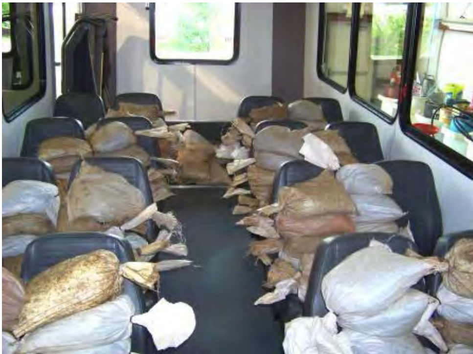
BUS LOADED TO 2.5 TIMES GVL (7,575 LBS)
