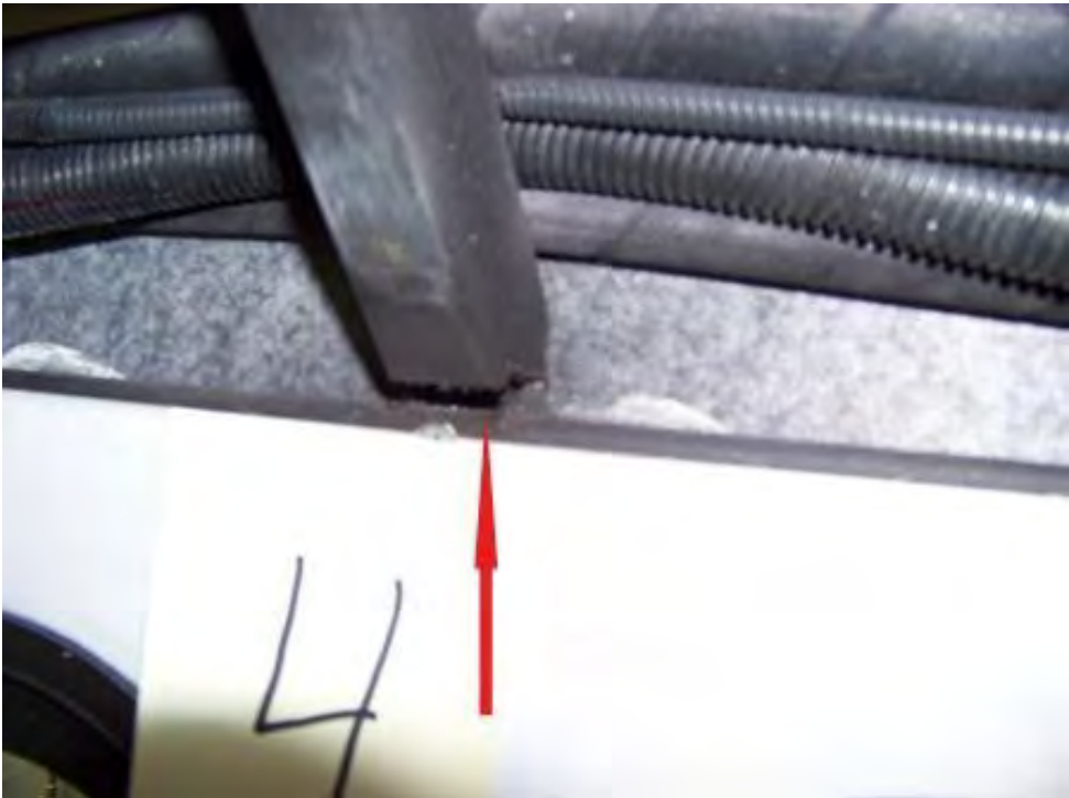
NUMEROUS (7) ROOF SUPPORTS ARE CRACKED OR BROKEN (6,846 TEST MILES)
