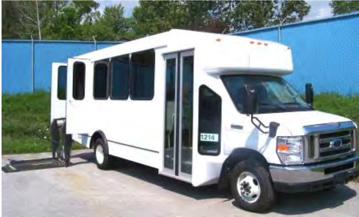
ELDORADO NATIONAL-KANSAS MODEL ADVANTAGE 240 EQUIPPED WITH A BRAUN MODEL L919F1B HANDICAP LIFT
