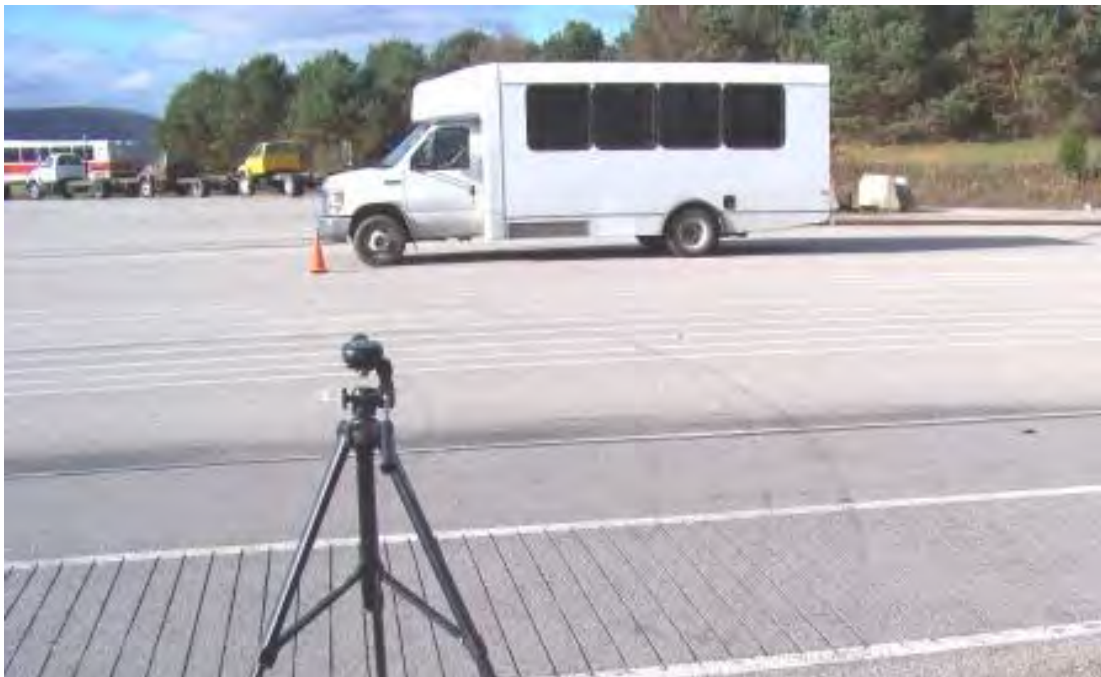
TEST BUS UNDERGOING EXTERIOR NOISE TESTING
