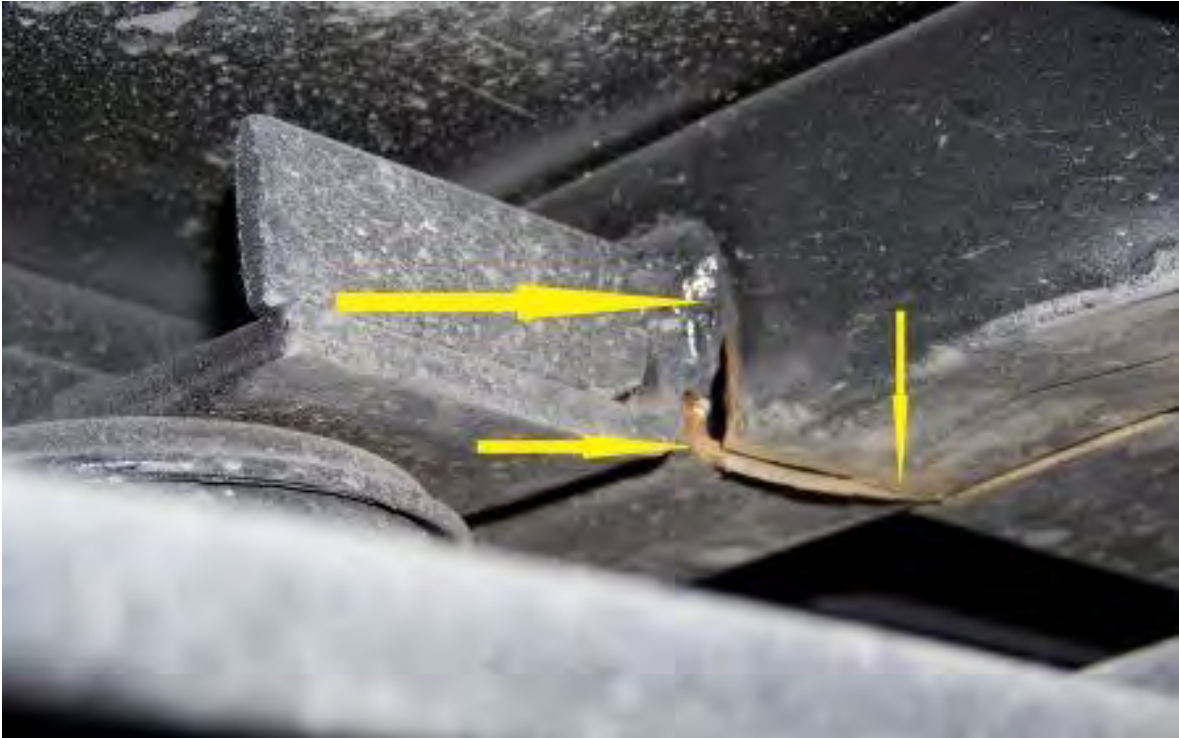
NUMEROUS FLOOR FRAME MEMBERS ARE CRACKED FORWARD & REAR OF THE REAR AXLE (2,171 TEST MILES)
