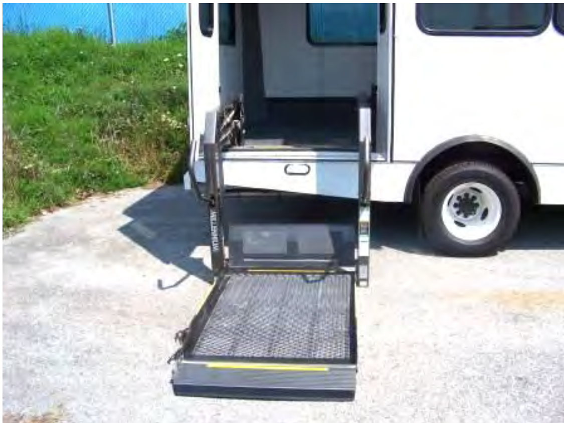
ELDORADO NATIONAL-KANSAS MODEL ADVANTAGE 240 EQUIPPED WITH A BRAUN MODEL L919F1B HANDICAP LIFT
