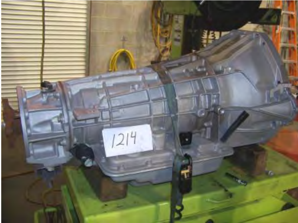
TRANSMISSION REMOVAL AND REPLACEMENT (8.00 MAN HOURS)
