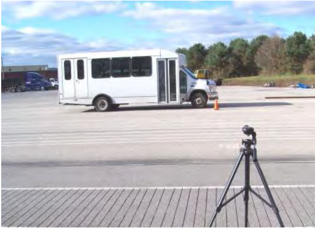
TEST BUS UNDERGOING EXTERIOR NOISE TESTING
