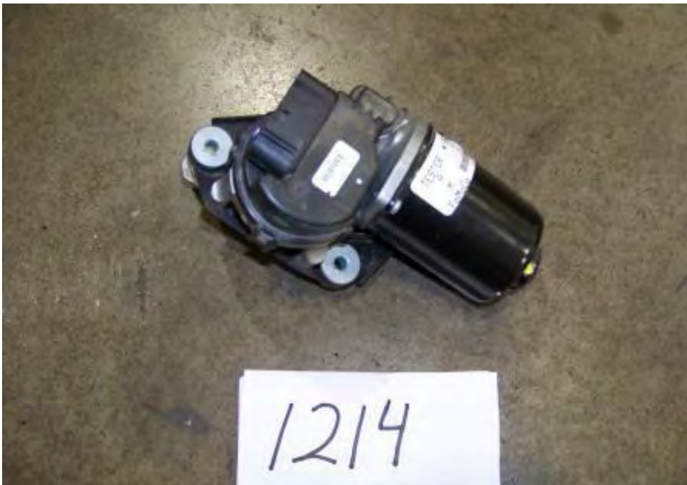
WIPER MOTOR REMOVAL AND REPLACEMENT (0.50 MAN HOURS)
