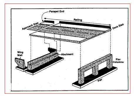
**Bridge pier or abutment** (Code 25): The walls or columns that support a bridge structure. (Abutments support the bridge ends, piers are the intermediate supports.) Collisions with these objects will normally involve vehicles traveling under bridges.
