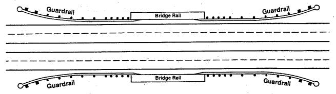
**Guardrail:** A barrier placed lengthwise along the edge of the roadway for the purpose of protecting a vehicle that strays from its intended path from striking a hazard, and redirecting it towards the roadway. The type of guardrail used in Nebraska is usually steel beam or cable. The guardrail codes used for First Harmful Event are broken down into two categories:
