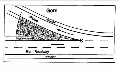
Code '7,' "Gore," should be used for accidents where the "First harmful event" occurs at a roadway gore. A gore is the area, often triangular in shape, where two roadways which carry traffic traveling in the same direction, come together or split apart. (See diagram)
