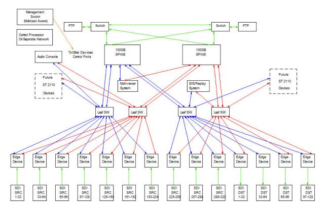
Detail must be provided in the response describing how vendor will propose the new SMPTE 2110 router will integrate into a mobile live production truck environment. Routing system should have a topology similar to the diagram above. SDI total count will vary depending on final design. Detail should include items below:
