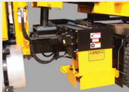
Front Cross Conveyor with Two Ply High-Temp Rubber Belting and Front Mounted Spinner
