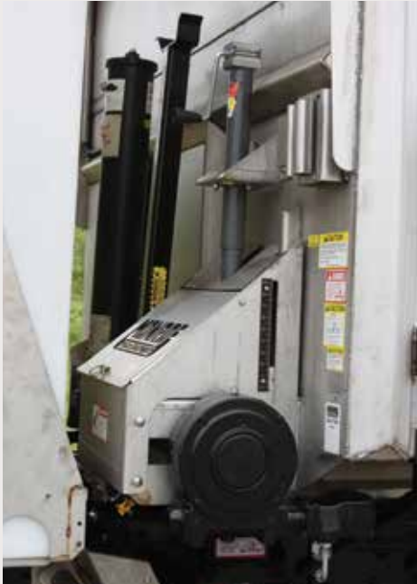
25:1 Drive System & Screw Adjustable Gate
