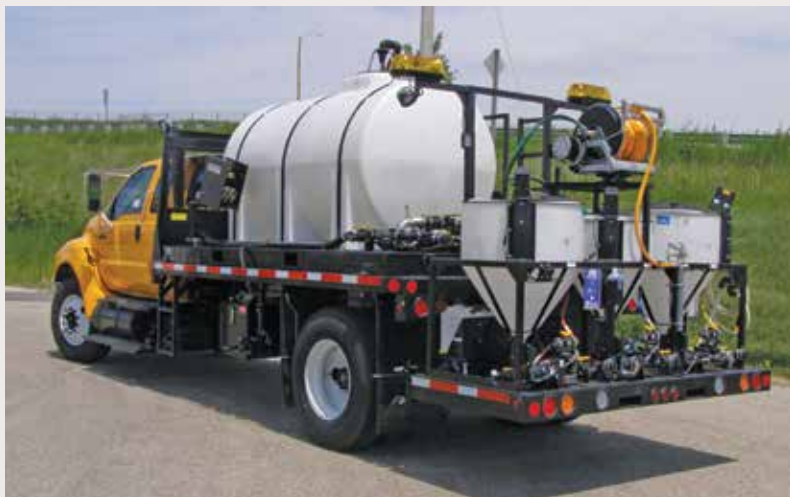
1000 Gallon System w/ Removable Skid
