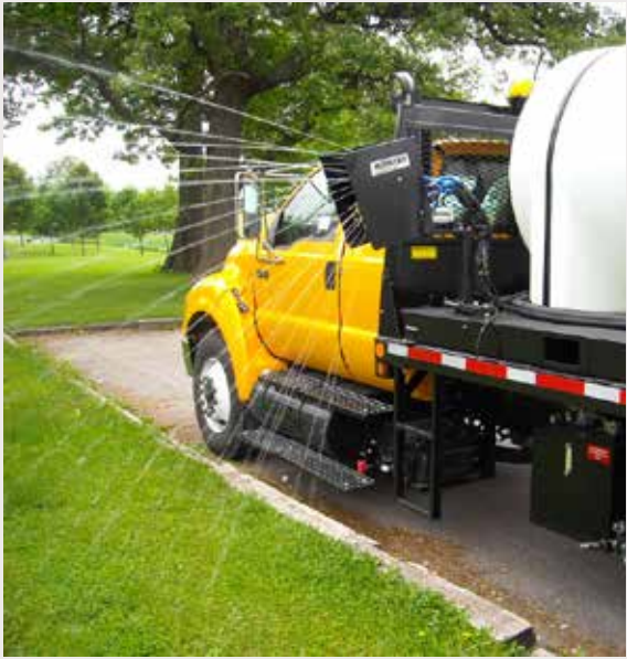
Spray Head: Front, Mid or Rear Mounted. Multi-Zone Spray Load with 30° Linear Actuation Tilt to Follow Ground Contour.
