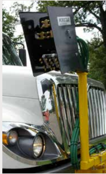
Guard Rail Underbody Spray Booms Manual or Power Height Adjustable Optional Spot Light Shown
