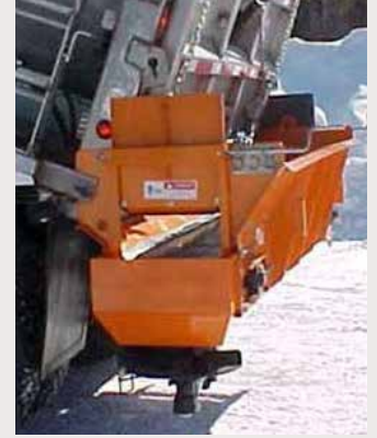
Rear Cross Conveyor
