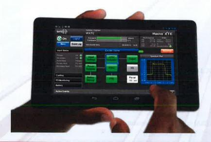
In addition to local control, the Maxiva ULXTE transmitter can be controlled from anywhere in the world with an intuitive, browser-based graphical user interface (GUI) over TCP/IP via a telecom or network connection with password protection. A rear RJ-45 jack is provided for LAN/WAN connection.
