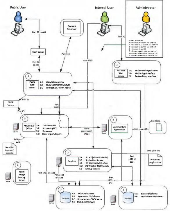
The figure below represents a logical network diagram illustrating the various application components and communication ports used by the system.
